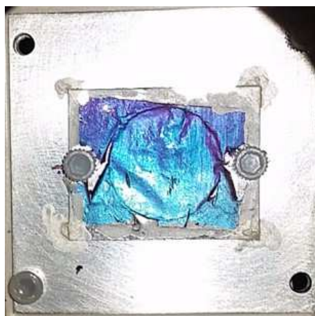
FIGURE 6.21: Photograph of ^{28}\text{Si} target foil mounted to a frame.
